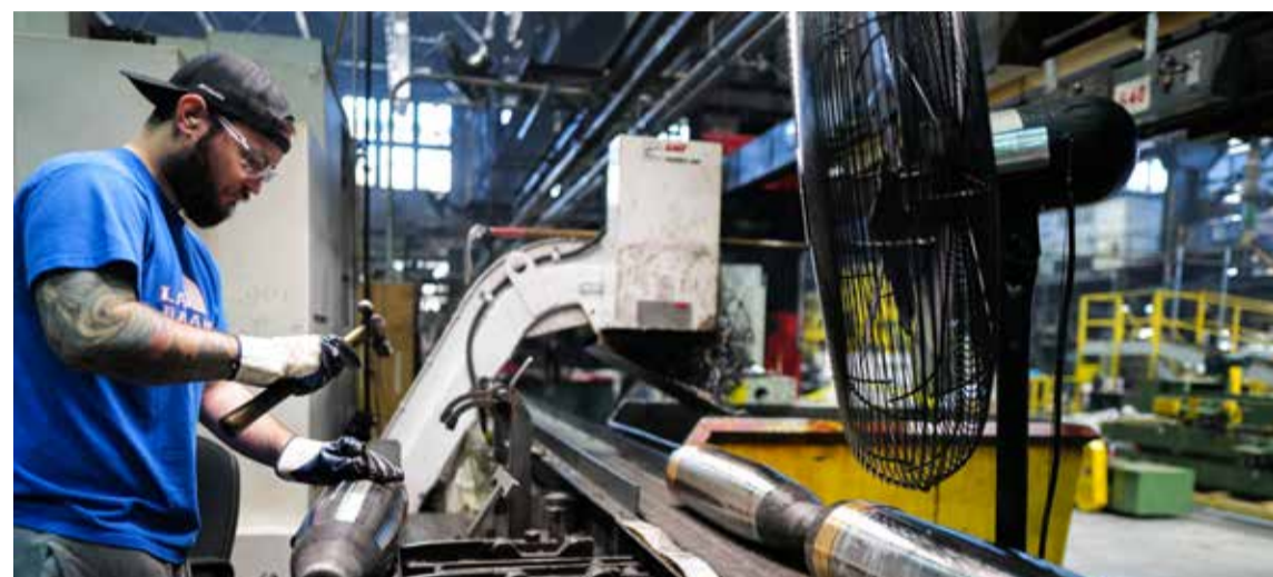
SCRANTON: An employee checks 155 mm caliber shells after the manufacturing process at the SCAAP in Scranton, Pennsylvania.
